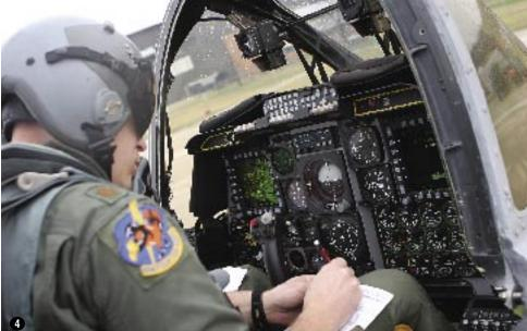
[3] Renowned for its versatility, the A-10 offers 11 hardpoints for carriage of fuel or weapons. [4] Maj. Eric Murphy in the A-10's front office. Many of the analog steam gauges have been replaced with color displays and computers as part of the precision engagement upgrade.
